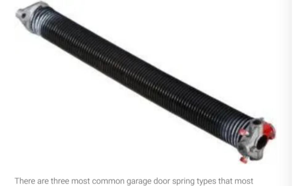
garage door manufacturers use. Torsion springs, extension springs, and a Torquemaster spring system. Torsion springs are by far the most common springs here in Canada and most likely worldwide. Most standard residential torsion springs are rated for about 10 -12 thousand cycles and will last on average 7 - 10 years, providing you with the smooth operation of your garage door. When balanced properly, your garage door should be very light, and most
