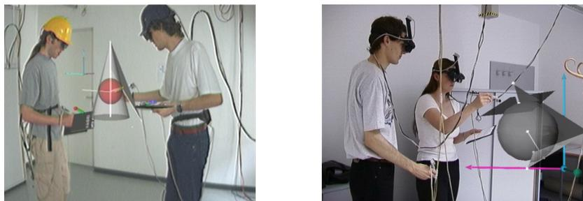
**Figure 1:** Students are working with Construct3D in our standard lab setup. In the left image they inscribe a sphere in a cone, the right image shows a simple example from vector algebra. Images generated as live video capture with computer overlays.
